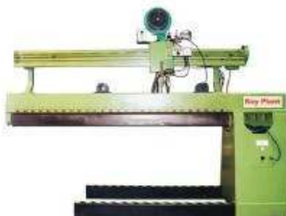
2500 mm Seam Welder set up for Mig Welding.
