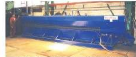
6500mm Seam Welder set up for Sub Arc Welding.
