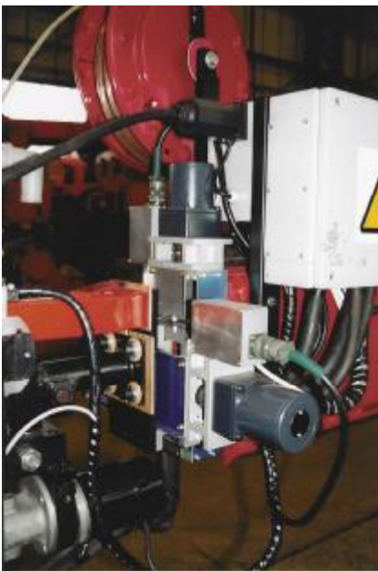
Model Type – SGD215CL with 150mm of stroke.
