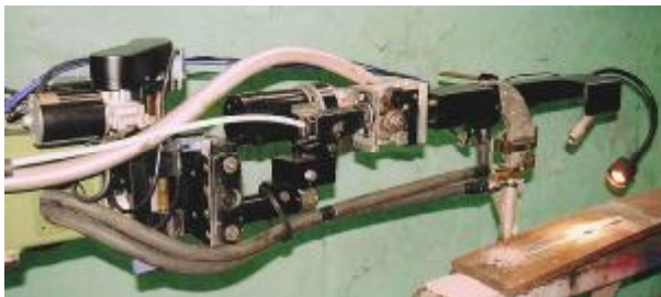
Internal welding head to weld inside 300mm pipe fitted with a camera
