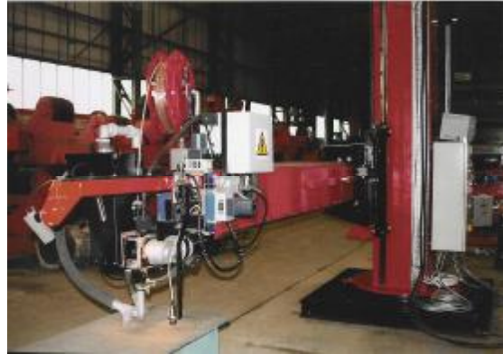
A column & boom welding installation
