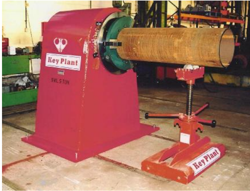
Photograph shows : Hollow Bore 5 Ton Headstock with Adjustable Height Idler
